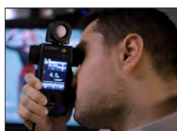
Accurate targeting of a subject is quick with the SLR designed 1 deg Spot lens. For ease of use the eye piece provides an adjustable diopter for sharp viewing.
